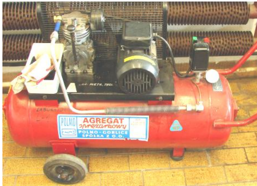
Fig 5 Compressor installation as a measurement position
